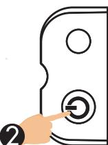
Press and hold the on / off button of the TV RCU. Wait until the red light on the NEXT RCU is steady. When the light is steady, this key is programmed to the NEXT RCU
