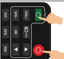
Press and hold the Green and Red on/off buttons from the Next Digital controller simultaneously for 5 seconds. When the red light is steady, stop pressing. Next Digital remote controller is now in learning mode.
