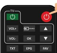
After the programming process is finished, press the red on / off button on the NEXT Digital RCU to save. You can now control your TV with the buttons in the TV area.
